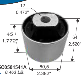
BUJE BRAZO SUSPENSION TRASERA REAR SUSPENSION CONTROL ARM BUSHING
