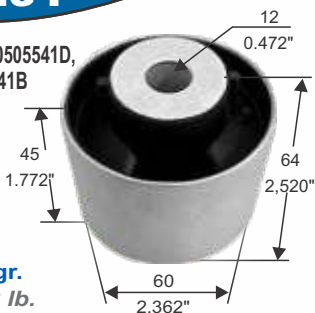
BUJE GRANDE BRAZO SUSPENSION TRASERA REAR SUSPENSION CONTROL ARM BUSHING
